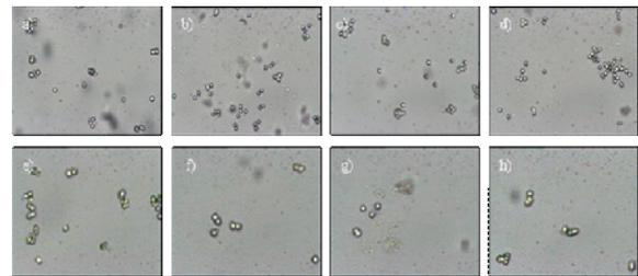
Fig. 7: Microstructure of DCA microspheres in different periods at initial state (a), 24 hours (b), 9 days (c), 30 days (d), 60days (e), 90 days (f), 120 days (g) and 180 days (h).
