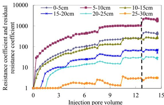
Fig. 9: Resistance coefficient and residual resistance coefficient change with PV each measurement point.
