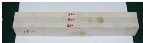
Fig. 3: The size of three layers of heterogeneous artificial core: 30 cm×4.5 cm×4.5cm.
