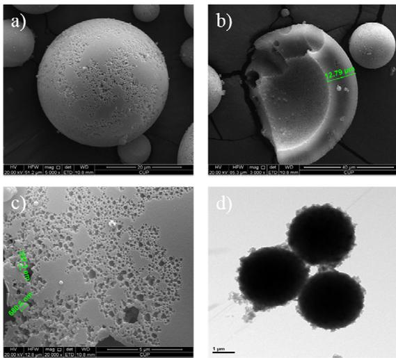
Fig. 5: External structure (a), internal structure (b) and external microstructure (c) of DCA microspheres. Microstructure of DCA microspheres in water (d).
