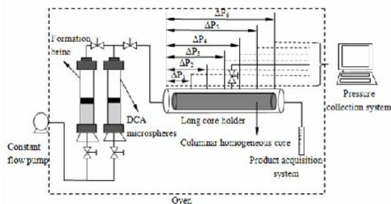
Fig. 2: Experimental flow chart of injection and plugging ability.
