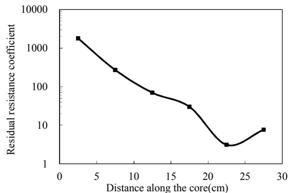
Fig. 10: Residual resistance coefficient change with the distance along the core.
