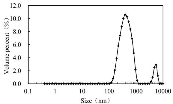
Fig. 8: Diameter distribution of the DCA microsphere.
