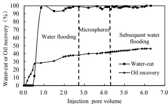
Fig. 11: Plugging effect of the DCA microspheres.
