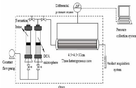
Fig. 4: Experimental flow chart of evaluation of plugging effect of DCA microsphere.
